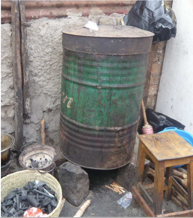
Figure 5 : Metal sheet smoking oven The smoke passes over the product
