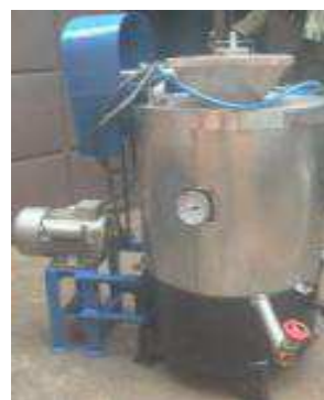
Mixer-cooker: equipment adapted to control the parameters during different steps (pasteurization, fermentation, cooking)
